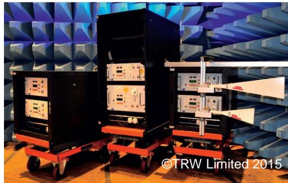
*TMD has its headquarters in Hayes, West London, and (right) a suite of its TWTAs in an HIRF testing facility.
